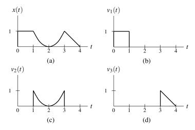
Figure 2.25: Representing piecewise polynomial function using unit-step functions.
