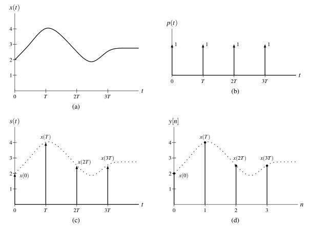
Figure 5.25: The various signals involved in the sampling process. (a) The original continuous-time signal x(t). (b) The sampling function p(t). (c) The impulse-modulated signal s(t). (d) The discrete-time signal y[n].
