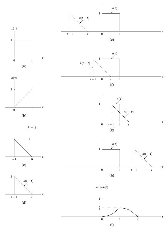
Figure 3.2: Evaluation of the convolution integral. The (a) input signal  $x(\tau)$ , (b) impulse response  $h(\tau)$ , (c) time-reversed impulse response  $h(-\tau)$ , and (d) impulse response after time-reversal and time-shifting  $h(t-\tau)$ . The functions associated with the product in the convolution integral for (e) t < 0, (f)  $0 \le t < 1$ , (g)  $1 \le t < 2$ , and (h)  $t \ge 2$ , (i) The convolution result x(t) \* h(t).
