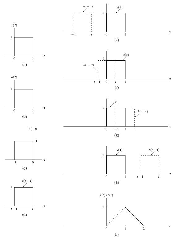
Figure 3.6: Evaluation of the convolution integral. The (a) input signal  $x(\tau)$ , (b) impulse response  $h(\tau)$ , (c) time-reversed impulse response  $h(-\tau)$ , and (d) impulse response after time-reversal and time-shifting  $h(t-\tau)$ . The functions associated with the product in the convolution integral for (e) t < 0, (f)  $0 \le t < 1$ , (g)  $1 \le t < 2$ , and (h)  $t \ge 2$ , (i) The convolution result x(t) \* h(t).
