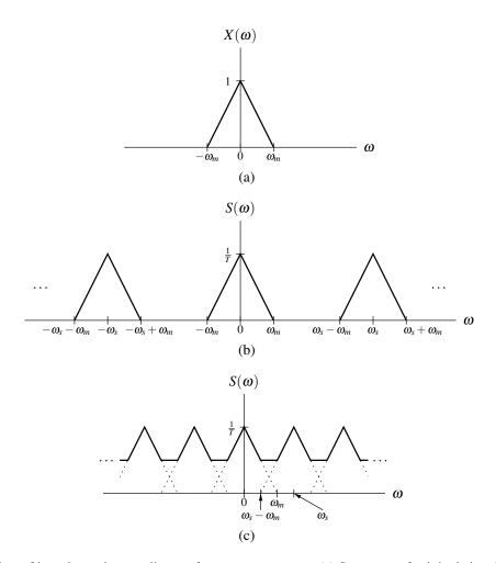
Figure 5.26: Effect of impulse-train sampling on frequency spectrum. (a) Spectrum of original signal x(t). (b) Spectrum of s(t) in the absence of aliasing. (c) Spectrum of s(t) in the presence of aliasing.
