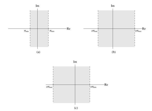
Figure 6.9: Regions of convergence for time-domain/Laplace-domain scaling. (a) Before scaling. After scaling for (b) a > 0 and (c) a < 0.
