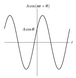
Figure 2.11: Real sinusoidal signal.
