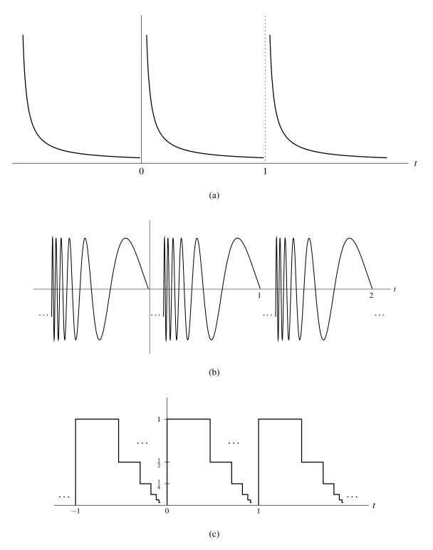
Figure 4.5: Examples of signals that violate the Dirichlet conditions. (a) A signal that is not absolutely integrable over a single period. (b) A signal that has an infinite number of maxima and minima over a single period. (c) A signal that has an infinite number of discontinuities over a single period.
