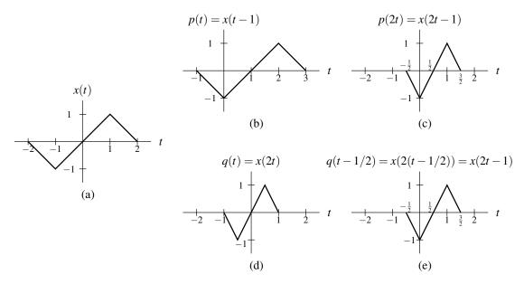
Figure 2.4: Two different interpretations of combined shifting and scaling transformation. (a) Original signal. Results obtained by shifting followed by scaling: (b) intermediate result and (c) final result. Results obtained by scaling followed by shifting: (d) intermediate result and (e) final result.
