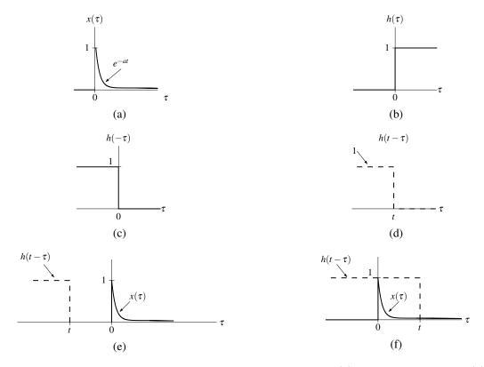
Figure 3.4: Evaluation of the convolution integral. The (a) input signal  $x(\tau)$ , (b) impulse response  $h(\tau)$ , (c) time-reversed impulse response  $h(-\tau)$ , and (d) impulse response after time-reversal and time-shifting  $h(t-\tau)$ . The functions associated with the product in the convolution integral for (e) t < 0 and (f) t > 0.
