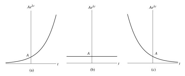
Figure 2.12: Real exponential signal for (a)  $\lambda > 0$ , (b)  $\lambda = 0$ , and (c)  $\lambda < 0$ .
