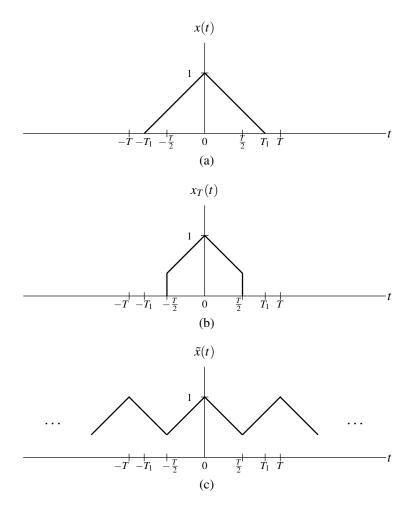
Figure 5.1: Example of signals used in derivation of Fourier transform representation (where  $T_1 > \frac{T}{2}$ ).
