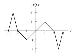
Figure 2.8: Example of an odd signal.
