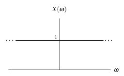
Figure 5.7: Frequency spectrum of the unit-impulse function.
