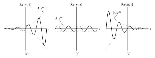
Figure 2.14: Real part of a general complex exponential for (a)  $\sigma > 0$ , (b)  $\sigma = 0$ , and (c)  $\sigma < 0$ .
