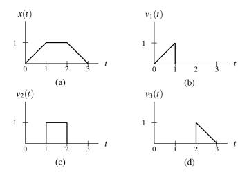
Figure 2.24: Representing piecewise linear function using unit-step functions.
