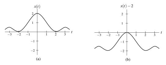
Figure 2.6: Example of amplitude shifting.
