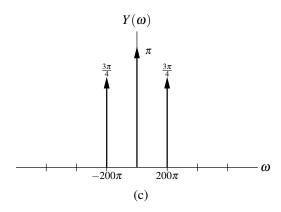
Figure 5.19: Frequency spectra for lowpass filtering example.
