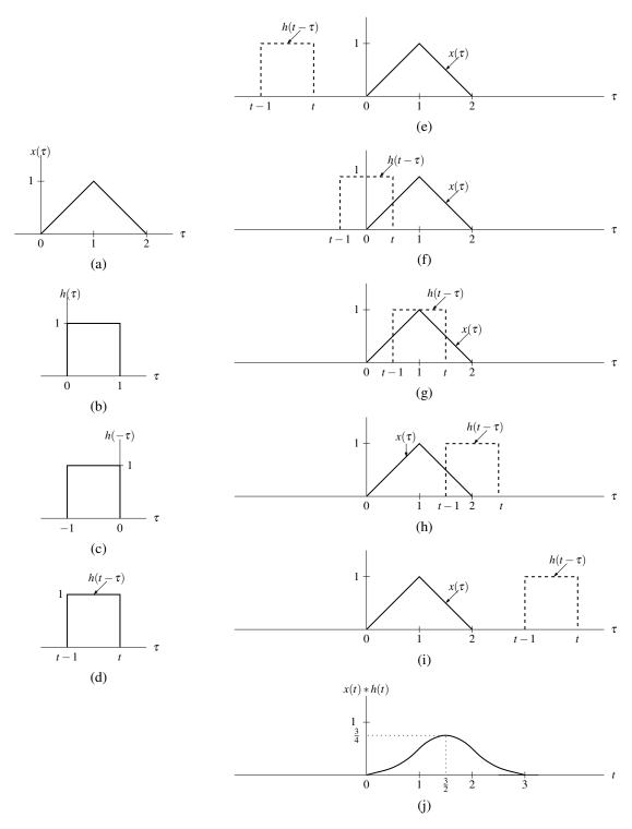
Figure 3.3: Evaluation of the convolution integral. The (a) input signal  $x(\tau)$ , (b) impulse response  $h(\tau)$ , (c) time-reversed impulse response  $h(-\tau)$ , and (d) impulse response after time-reversal and time-shifting  $h(t-\tau)$ . The functions associated with the product in the convolution integral for (e) t < 0, (f)  $0 \le t < 1$ , (g)  $1 \le t < 2$ , (h)  $2 \le t < 3$ , and (i)  $t \ge 3$ . (j) The convolution result x(t) \* h(t).
