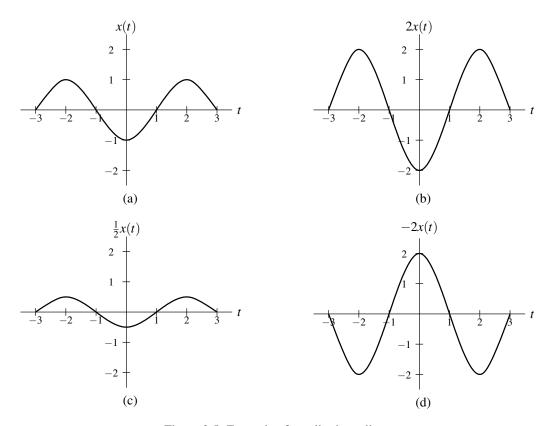
Figure 2.5: Example of amplitude scaling.
