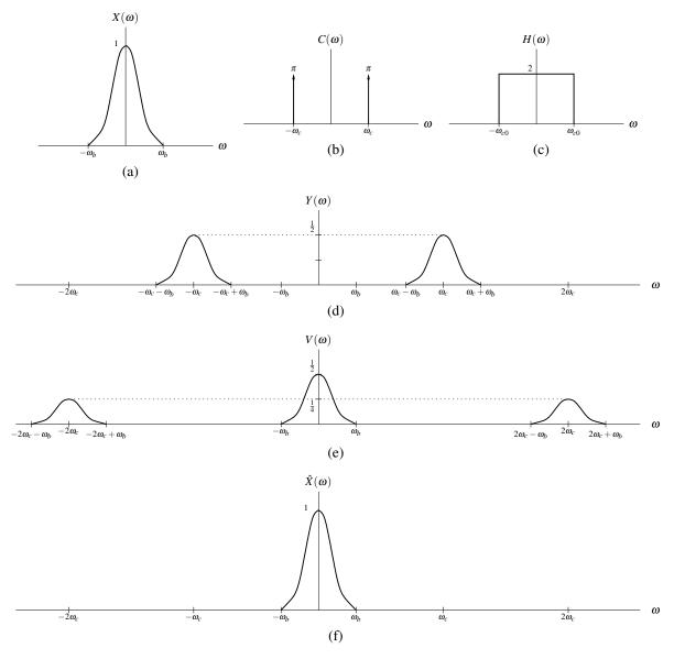
Figure 5.33: Signal spectra for DSB/SC amplitude modulation.
