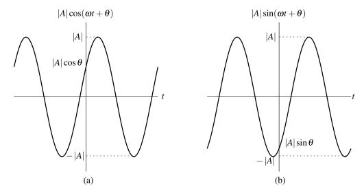
Figure 2.13: Complex sinusoidal signal. (a) Real and (b) imaginary parts.
