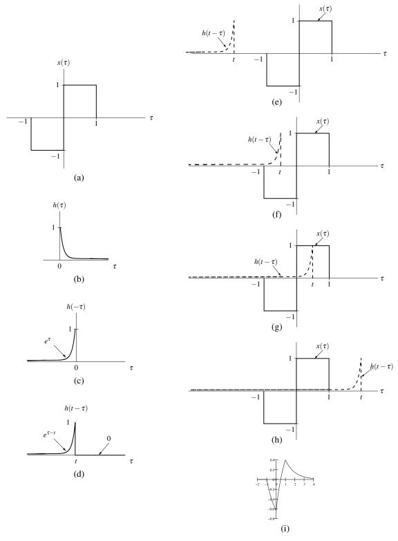
Figure 3.1: Evaluation of the convolution integral. The (a) input signal  $x(\tau)$ , (b) impulse response  $h(\tau)$ , (c) time-reversed impulse response  $h(-\tau)$ , and (d) impulse response after time-reversal and time-shifting  $h(t-\tau)$ . The functions associated with the product in the convolution integral for (e) t < -1, (f)  $-1 \le t < 0$ , (g)  $0 \le t < 1$ , and (h)  $t \ge 1$ , (i) The convolution result x(t) \* h(t).
