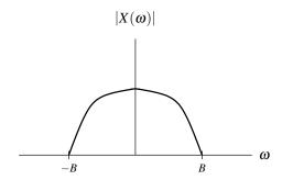
Figure 5.11: Bandwidth of a signal.
