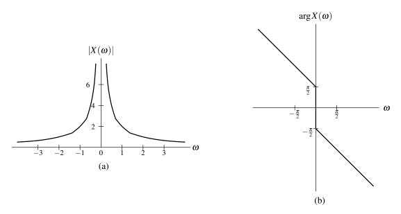
Figure 5.6: Frequency spectrum of the time-shifted signum signal. (a) Magnitude spectrum and (b) Phase spectrum.
