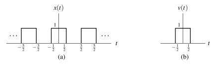
Figure 2.26: Representing periodic function using unit-step functions.
