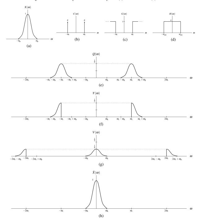
Figure 5.35: Signal spectra for SSB/SC amplitude modulation.
