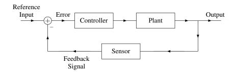
Figure 1.7: Feedback control system.
