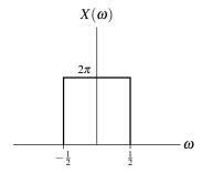
Figure 5.8: Frequency spectrum of the sinc function.
