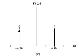
Figure 5.20: Frequency spectra for bandpass filtering example.
