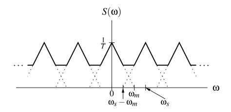
Spectrum of Impulse-Sampled Signal: Aliasing Case  $(\omega_s \leq 2\omega_m)$
