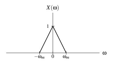
Spectrum of Input Signal (Bandwidth  $\omega_m$ )
