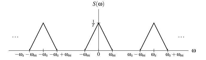
Spectrum of Impulse-Sampled Signal: No Aliasing Case  $(\omega_s > 2\omega_m)$
