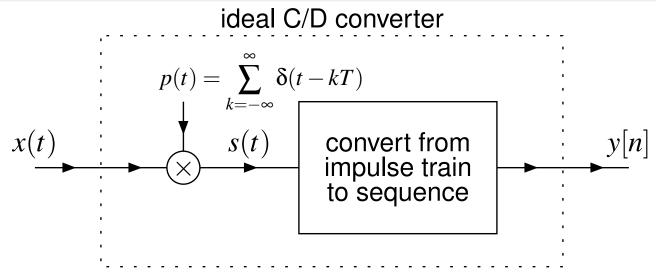
ullet In the time domain, the impulse-sampled signal s(t) is given by
