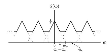
Spectrum of Impulse-Sampled Signal: Aliasing Case  $(\omega_s \leq 2\omega_m)$
