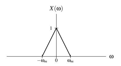
Spectrum of Input Signal (Bandwidth  $\omega_m$ )
